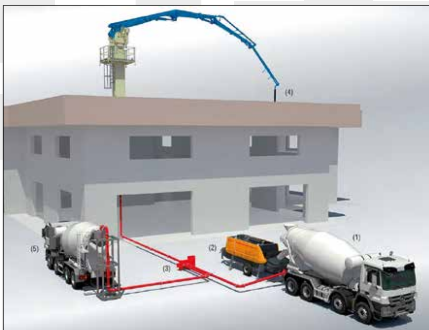
Figure 11. Operating mode and integral parts of stationary concrete pump: 1. truck mixer for concrete delivery, 2. stationary pump; 3. shutter regulating flow; 4. concrete spreader; 5. truck mixer for return of concrete
